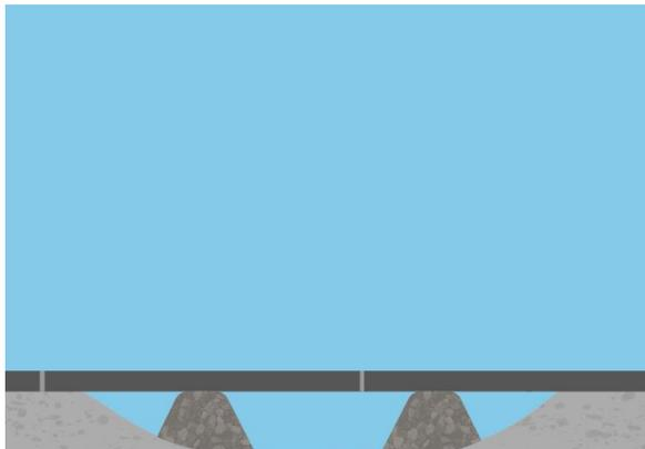
*To reduce excessive static stress on the pipeline, rock material will be used to reduce the length of freespans.*
