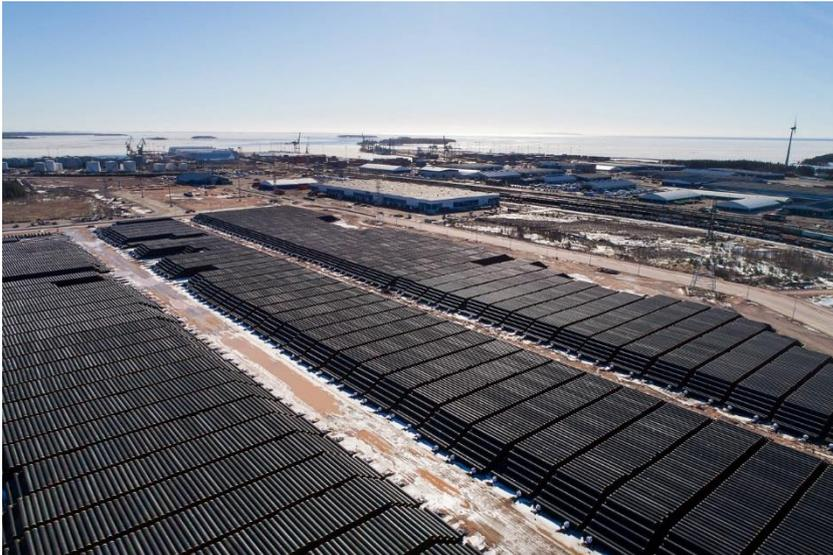
*Picture: Over 35,000 pipes are waiting to be concrete weight coated at Wasco's storage yard in Kotka, Finland. (© Nord Stream 2 / Wolfram Scheible)*
