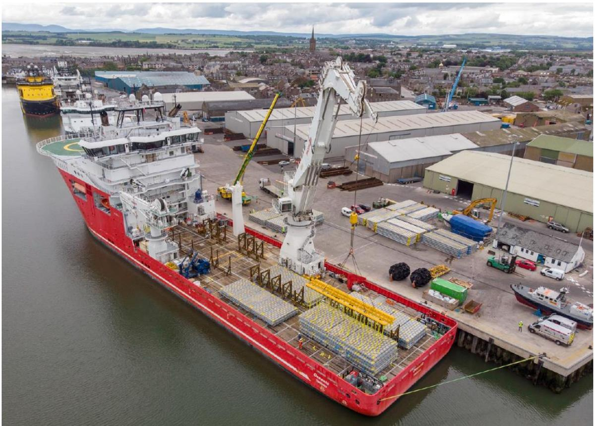
*Concrete mattresses being up-loaded to vessel Oceanic performing the mattress installation works.*
