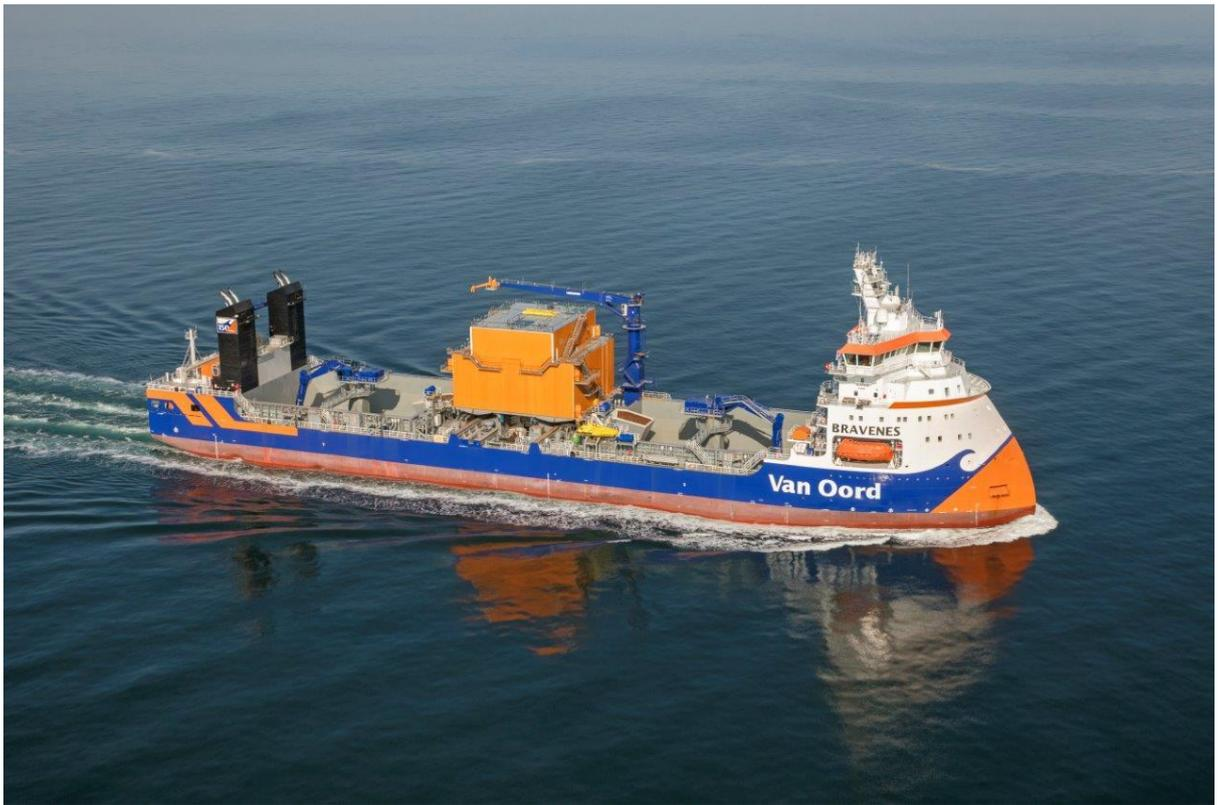
*Bravenes, one of the state-of-the-art fallpipe vessels, used for the rock placement (Photo: Van Oord).*
